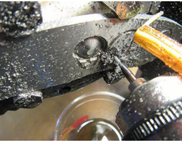
▲ Figure 2: 3D profiling a handle liner on the Pocket NC, image courtesy of Duncan Custom Knives
